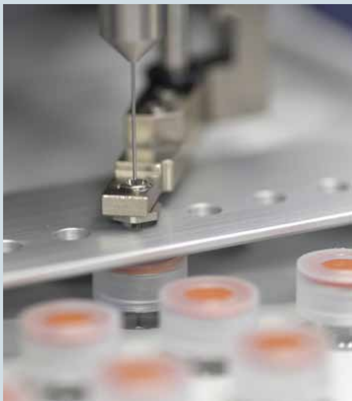
Heated nozzle of the ATS 4 (option)
