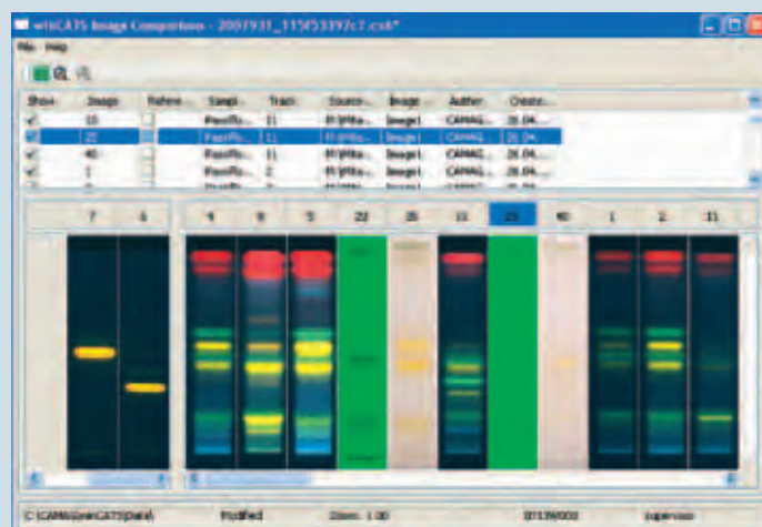
Image Comparison View: Selected tracks of images taken of the same plate under UV 254 nm (20, 25), white light (35, 40) and UV 366 nm (all other tracks) are compared
